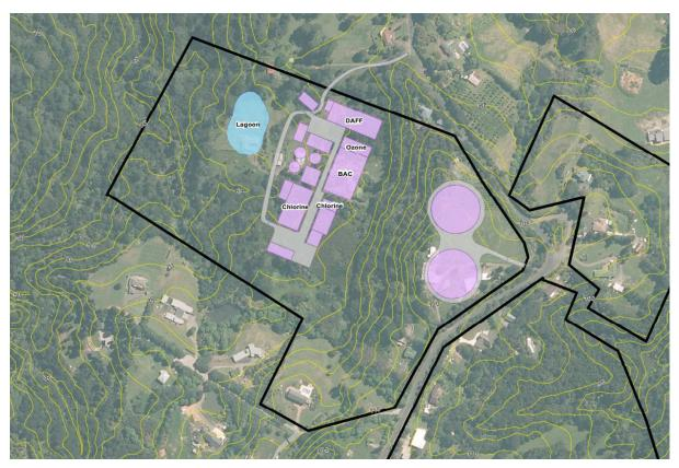
Figure 4.5: Upper Carter scheme concept layout, captured from GHD Drawing "Figure 1, Huia WTP Site Selection Study Preliminary Site Layouts, Site: 51 – Carter 1", Job Number 51-33575, Revision 0, dated 14 December 2015
